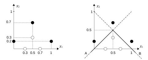
They can be separated, instead, by a piece-wise linear boundary made up of two half-lines, like the ones denoted by A and B in the figure above in the middle. This means that a consistent solution can be obtained by a feed-forward multi-layer perceptron network with one hidden layer made up of two hidden units (see figure below), whose activations correspond to the equations of line A:  $x_2 = x_1$ , and of line B:  $x_2 = 1 - x_1$ .
