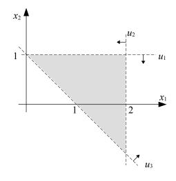
It is easy to see that the output unit implements the AND Boolean function between the outputs of the hidden units. Therefore the region where the network output equals 1 is the shaded area in the figure above; outside this region the network output equals 0.
